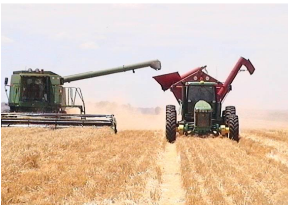
Photo 2 -catching hopper and cross auger on the chaser bin to allow unloading from the wheeltracks Source:www.precisionagriculture.com.au
