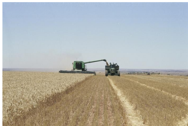
Photo 3 -Auger extended to allow unloading on the wheeltracks Source: DAFWA Webb et al 2004
