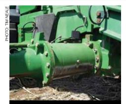
Axle extensions are one way to facilitate a move to CTF. The part pictured here was manufactured specifically for this tractor and while not as inexpensive as cotton reel spacings, it is a robust option that will not cause damage to the machine.
