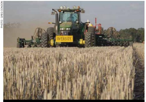
A gradual low-cost approach to machinery changeover was taken in this 9-metre system at Wagga Wagga, NSW. A Horwood Bagshaw seeder width was matched to the existing header, then axles on boom and spreader converted to 3m in the farm workshop. JD front wheel assist tractor on 3m is used for all operations. A new disc seeder was purchased in 2013 to complement the no-till continuous cropping and stubble retention system.
