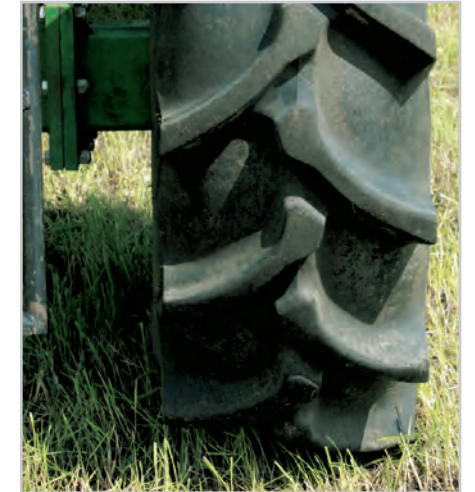
The rear wheel gauge on the air cart was extended to match the tramlines.
