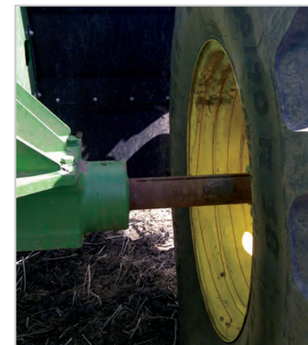
Equipment was set up on a 120-inch wheel gauge.
