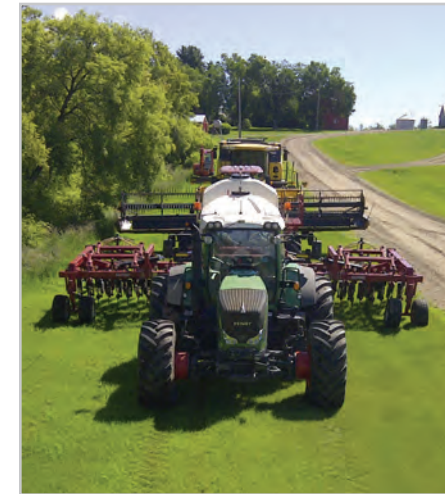
The CTF system was built on the 30-foot combine header width.
