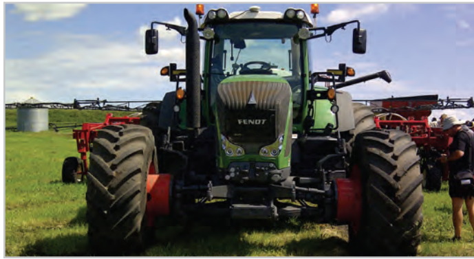
Wheel extensions for a 120-inch gauge.
