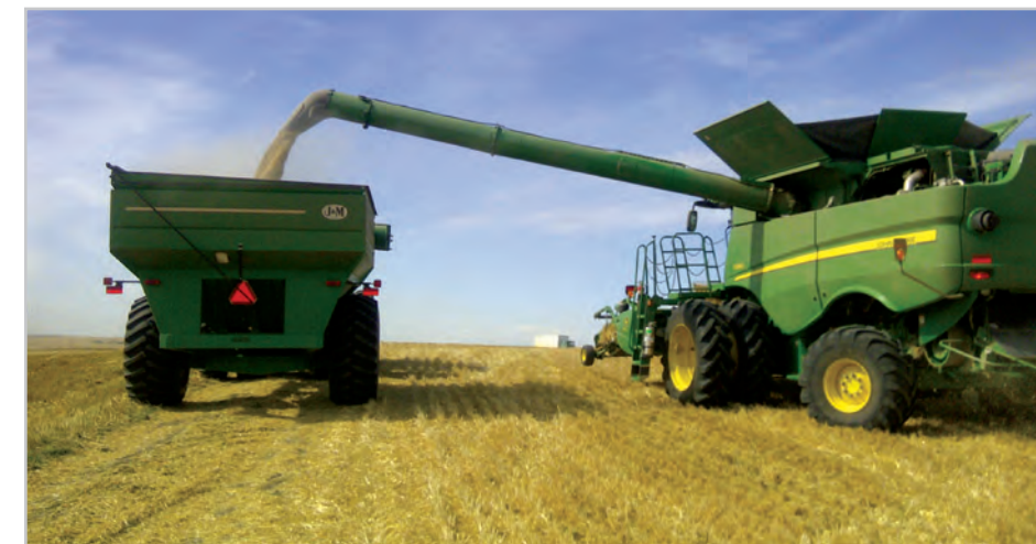
One challenge of the 40-foot system is having to move off the tramline to unload.
