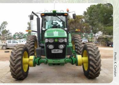
The John Deere 7730 spray tractor was adapted for 3 metre wheel tracks using cotton reel spacers in 2008.
