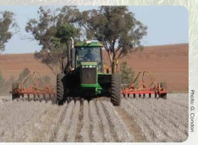
The inside wheels were removed from the duals on the sowing tractor to run on three metre wheel tracks. The seeder was reduced from 11 metres to 9 metres and row spacing widened to 333mm.
