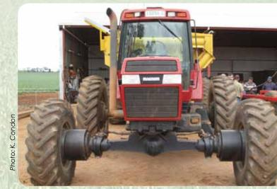
The wheels on the spreader were moved out to three metres to match the tractor. Although currently spreading to 18 metres (2:1), McKinleys plan to fit a new vane to allow urea to be spread to 27 metres (3:1).
