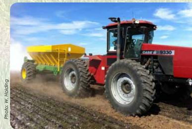
A Landaco belt spreader with three metre wheel base was recently purchased for lime, gypsum and urea applications. The inner wheels were removed from the Case tractor to match three metre tracks.
