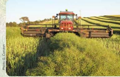
The self-propelled windrower is matched to the system and has vertical knives and a cross auger to allow even feeding of large windrows.
