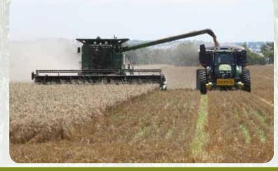
**Matching additional machinery:** An auger extension on this header in a 9-metre CTF system means the tractor and chaser bin are able to stay on the tracks during loading.
