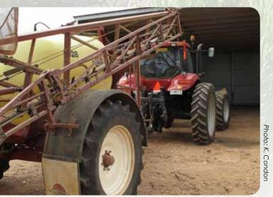
A Case front-wheel assist tractor on three-metre axles was purchased in 2009. The boomspray was widened to 24 metres in 2008, but they have since purchased a 36 metre boom (photo oppposite).
