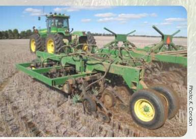
The John Deere single disc opener was widened to 10.67 metres and row spacing increased to 308mm for inter-row sowing. Aricks wheels were fitted to minimise hair pinning.
