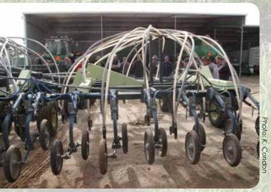
The 12-metre Alfarm airseeder is on 308mm row spacing with press wheels. Disc openers have been added for sowing wheel tracks, while disc coulters are used to cut through green manure residue.
