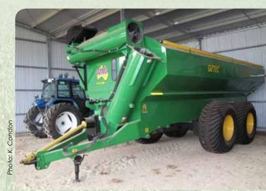
The Oztec chaser bin is on 3 metre, steerable axles. It is the only machine that runs off tracks during pick-up.
