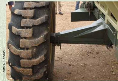
The axle was extended on the Marshall spreader in 2009 to suit three-metre wheel tracks.
