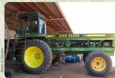
McKinleys recently converted a second-hand cotton picker into a 9-metre self-propelled windrower. Prior to 2011, the windrower was the only machine not matched to the system.
