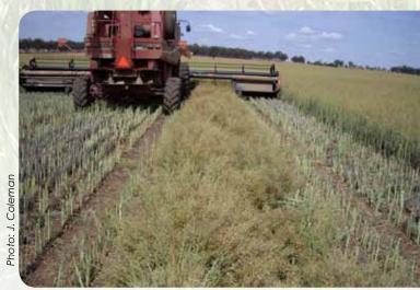
Although the windrower is not matched to the system, canola is windrowed using a 9 metre draper front with three metre offset so windrows are placed in the centre of the tracks.
