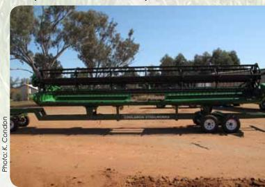
The new 9-metre centre mounted front is able to be used for both the header and self propelled windrower.
