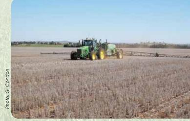
The boomspray was widened to 32 metres to match the 10.67-metre system (3:1), and the axles of both the boomspray and tractor were extended to three metres.
