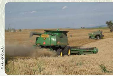
The header is fitted with a PowerCast™ tailboard for even straw distribution across the working width, essential to minimise hair pinning when disc seeding.
